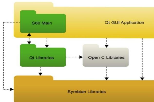
Figure 2: Architecture of Qt for Symbian <sup>[5]</sup>
