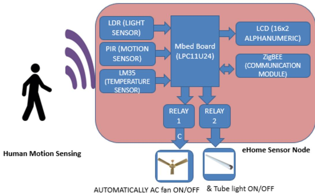
Fig 1: Architecture of sensor node
