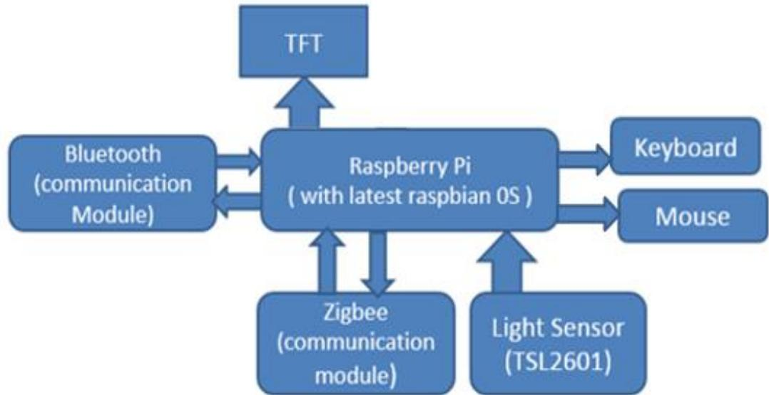
Fig 2: Architecture of gateway node
