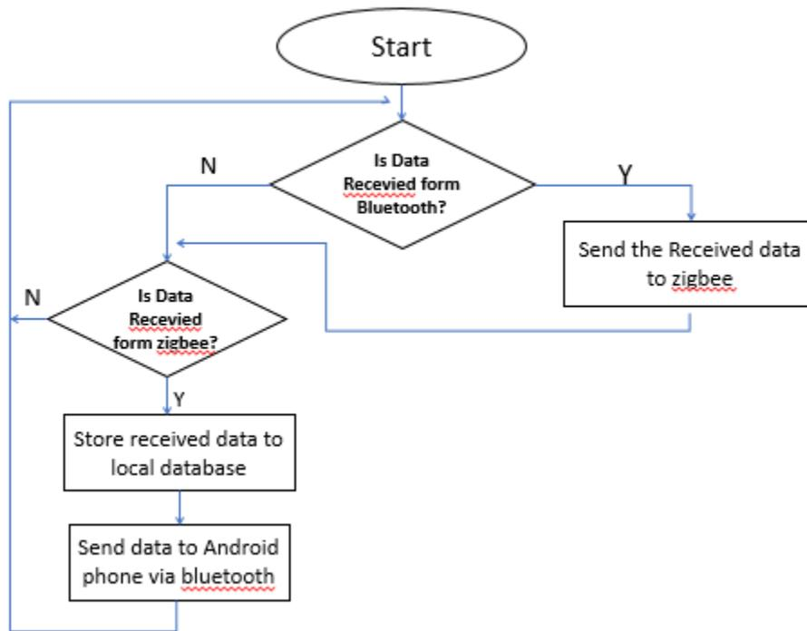
Fig 5: Flow chart of gateway node
