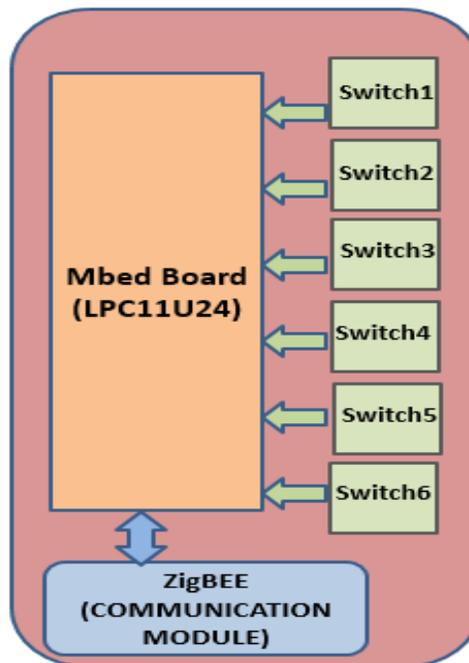
Fig 3: Architecture of control node
