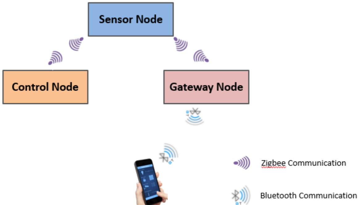
Fig 6: Network Architecture of sensor node
